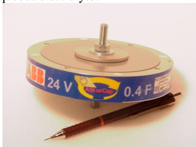
Figure 7: Super-capacitor for 5.7kW and an energy level of 115Joule.
